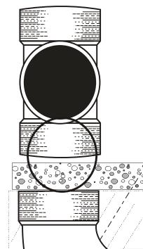
Because the water pressure may be as much as 30 lbs. (Or more), the possibility of a blow-out is very great, with the blow-up ball method. When this happens, the blow-up-ball is pushed down past the opening into the drain line. In order to retrieve the blow-up ball the pipe and concrete must be completely torn out and the ball located.
