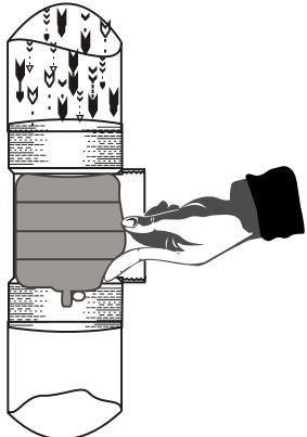
Our main competitor is the blow-up-ball, The inflatable, rubber ball is installed into the Test Tee Fitting, after the plumbing is complete.
